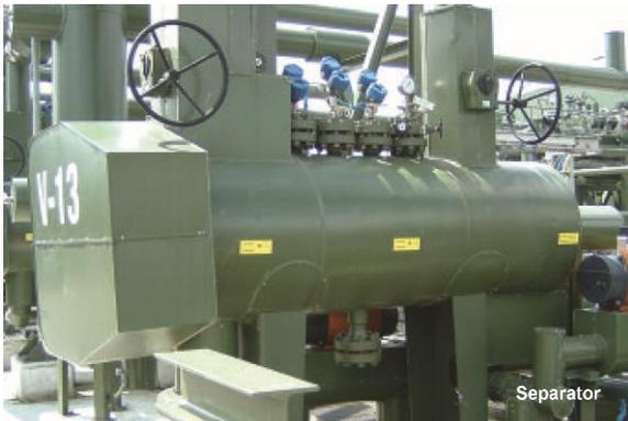
Separators are large drums designed to separate well streams into their individual components. They are designed to separate 2-phase (gas/liquid) or 3-phase (gas/crude/water) well streams.
