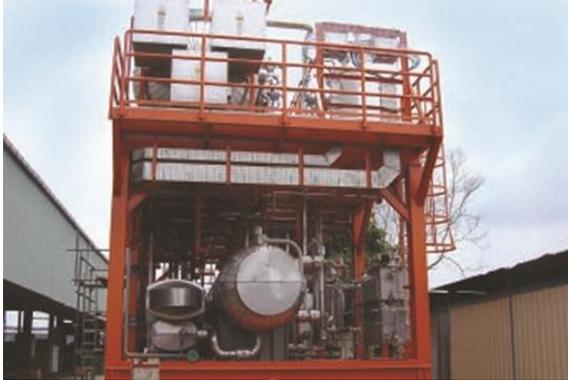
Natural Gas Dehydration removes hydrates which can grow crystals and plug lines and slow down flow of gaseous hydrocarbon streams. Dehydration also reduces corrosion, eliminates foaming, and prevents problems with catalysts
