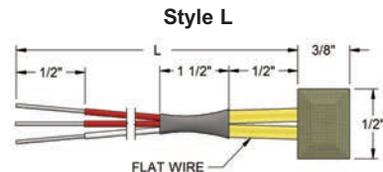
The JMS pad RTD is a specialty sensor which provides a fast response surface measurement. It is a 100Ω platinum RTD with an alpha of .00385 Ω/Ω°C. Pad material is PTFE (Teflon) impregnated glass fibre. The pad RTD has an effective operating range from -80°C to 200°C and its tolerance is 0.1Ω (± 0.26° C at 0° C). Additional Teflon leadwire is configured as a 3 wire RTD. High temperature configurations can be designed.
