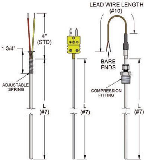
Note: L is the overall length of the sensor to the transition, wire, plug, head, or fixed attaching device. L excludes non-fixed attaching devices.
