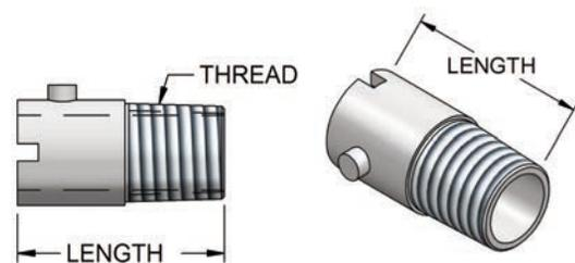
**NOTE:** To order adapters of different lengths, use 2A + X for 1/8" NPT and 2E + X for 3/8"-24 threads. You must specify length. Standard slot head adapters are nickel plated brass. Other materials are available upon request.
