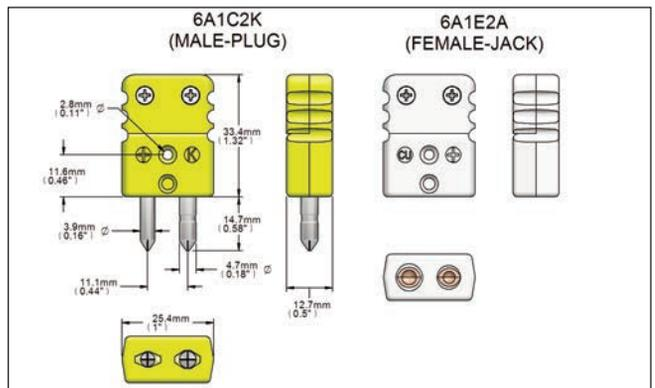
**Note:** Call JMS for high temp. vacuum applications and multi-pin connectors. Thermocouple plugs are normally two pin and RTD plugs are three pin. See page 6-4 for preferred RTD quick connectors.
