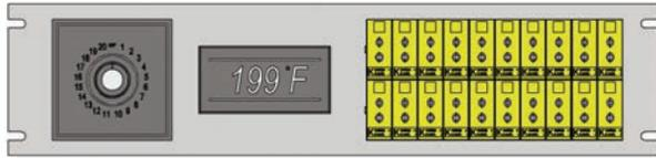
The JMS Deluxe Switch has an integral face plate and screw/solder terminals. Terminals are silver plated, brass numbered circuits w/ polarity identification. Blades and contacts are silver plated w/ self-cleaning wiper action. The "OFF" position has terminals available for shorting input circuit when using the switch w/ a digital meter. Order numbers 63-2 through 63-10 are break before make. Order numbers 63-12 through 65-40 and 6R-6 through 6R-36 are make before break.
