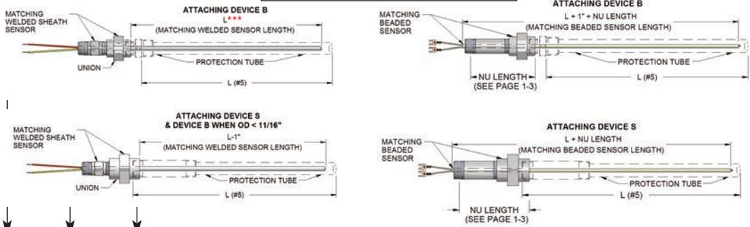
**Note: Do NOT use spring-loaded sensors in ceramic protection tubes.**
