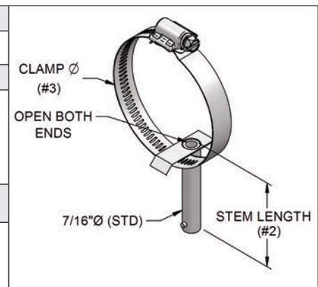
**Note:** L = Length of stem. Should be equal to the maximum insulation thickness + 3/4". The bayonet sensor length for adjustable should be L + 1-1/4". For fixed, it should be L + 1/2".
