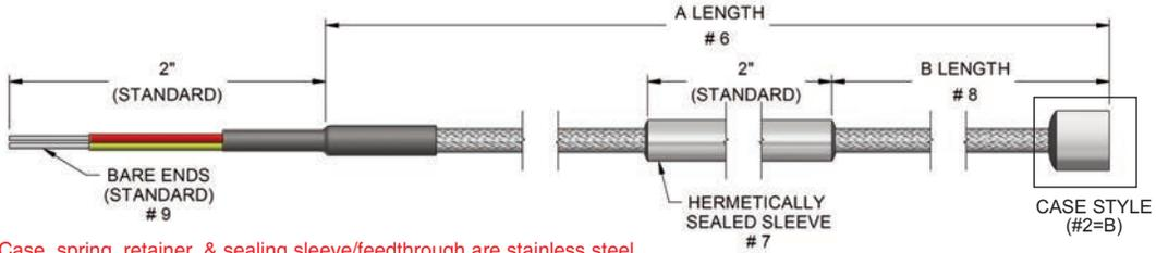
Note: Case, spring, retainer, & sealing sleeve/feedthrough are stainless steel.
