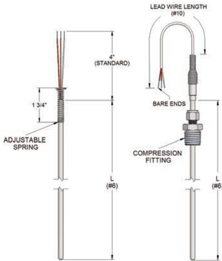
**Note:** L is the overall length of the sensor to the transition, wire, plug, head, or fixed attaching device. L excludes non-fixed attaching devices.
