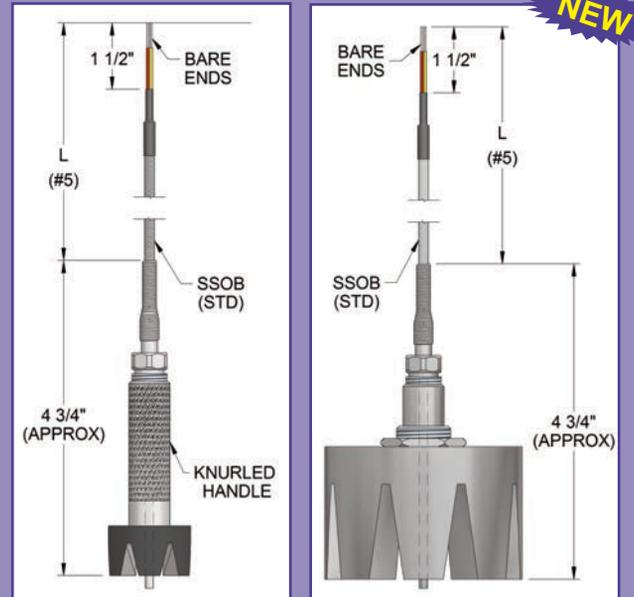
Note: Thermocouple wire is 24 AWG solid conductors. RTD wire is 24 AWG stranded conductors.
