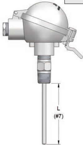
**Note:** L is the length of the sensor to the fixed attaching device.
