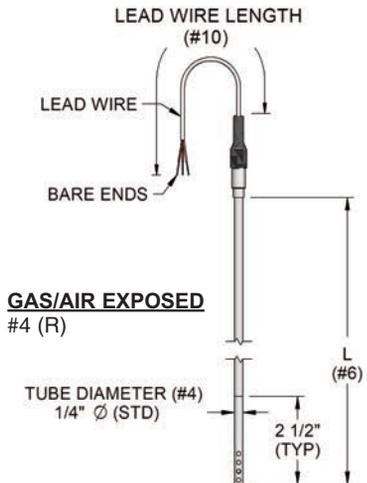
Note: Immersion shown (#6) is overall length of tube for gas air sensors.
